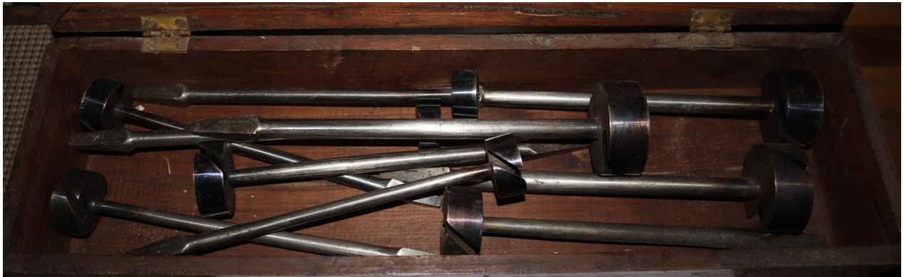
5. Set of large Forstner bits made by PM Co. (1 1/8 to 2")
