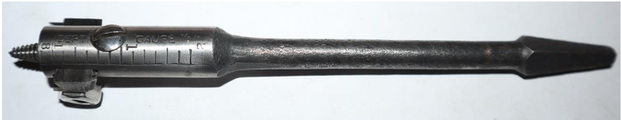
13. Irwin solid center long augers (without handles) Marked "IRWIN USA" vertical around shaft. Shown with 12" ruler as reference. Sizes T-B 28 (1 3/4"), 20 (1 1/4"), 9, 8.
